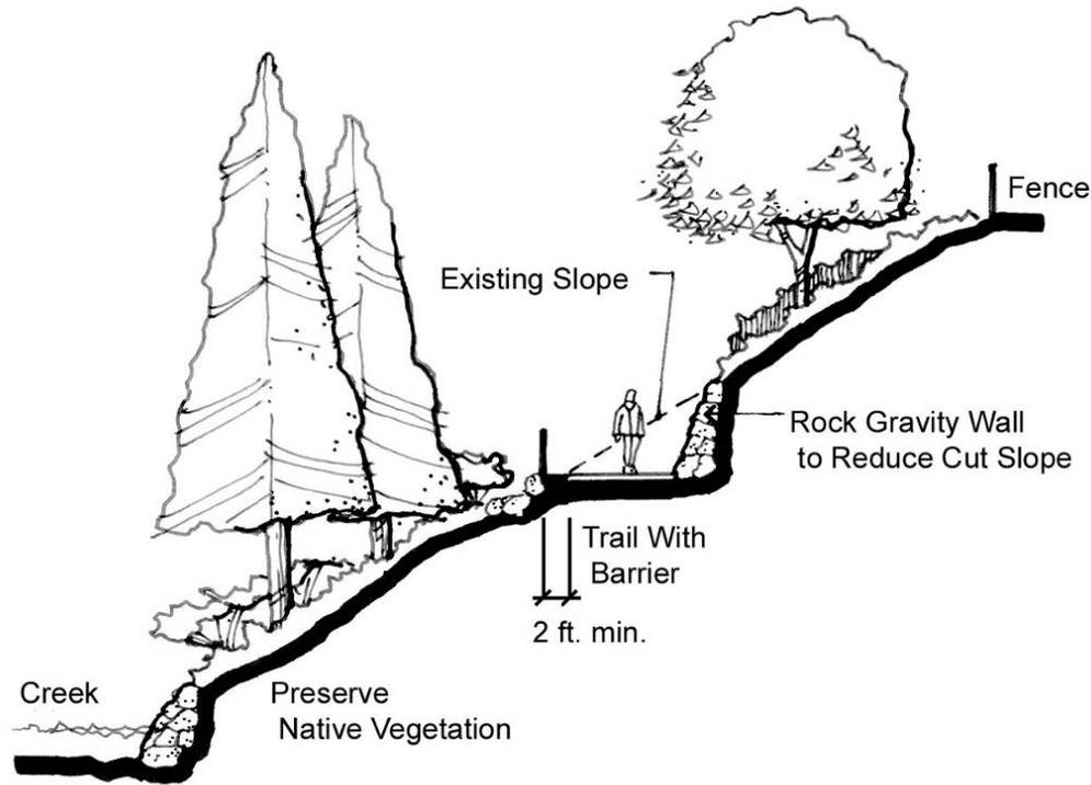
Figure 7 illustrates a typical soft surface trail design that is appropriate for foot trails in steep and inclined areas. This type of trail with a typical width of 3'-6' is designed to accommodate walkers, hikers and runners, depending on available space. The foot trail will be an earthen or other "soft" surface, so it is not appropriate for most bicyclists, nor will it meet ADAAG requirements. The trails should be designed with adequate drainage to prevent channeling and erosion.
