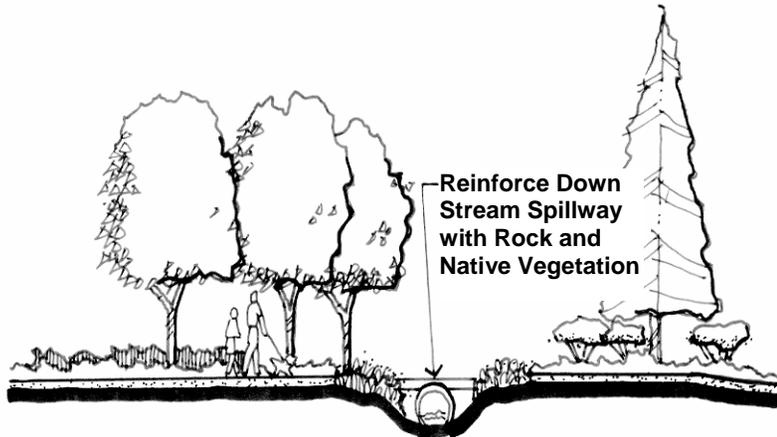
**Figure 13.** *Low Water Crossing of Minor Stream or Drainage*
